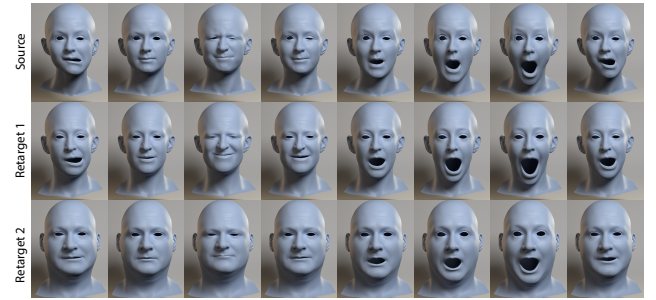
Figure 6: Our method allows to easily retarget performances from one individual (row 1) to any others (rows 2 and 3).
