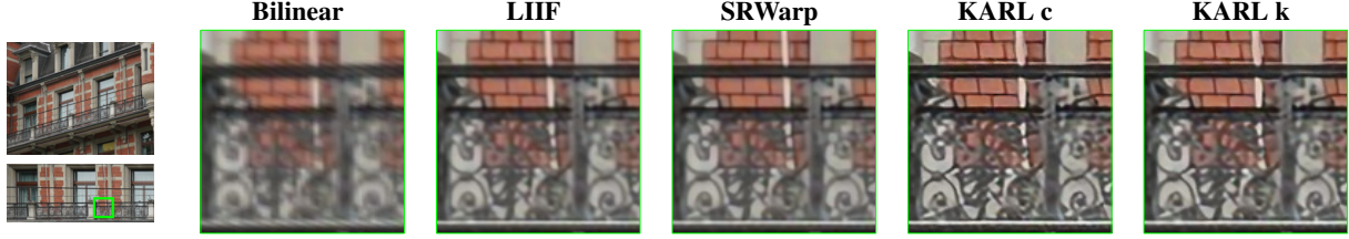
Figure 6. Comparison on real image rectification. The unknown kernel maps are estimated for the results generated by our method. We show the results both when predicting the output color directly (KARL c) and when predicting a 5 \times 5 kernel that is applied to the input image (KARL k). Both methods produce visually more appealing results than LIIF and SRWarp.
