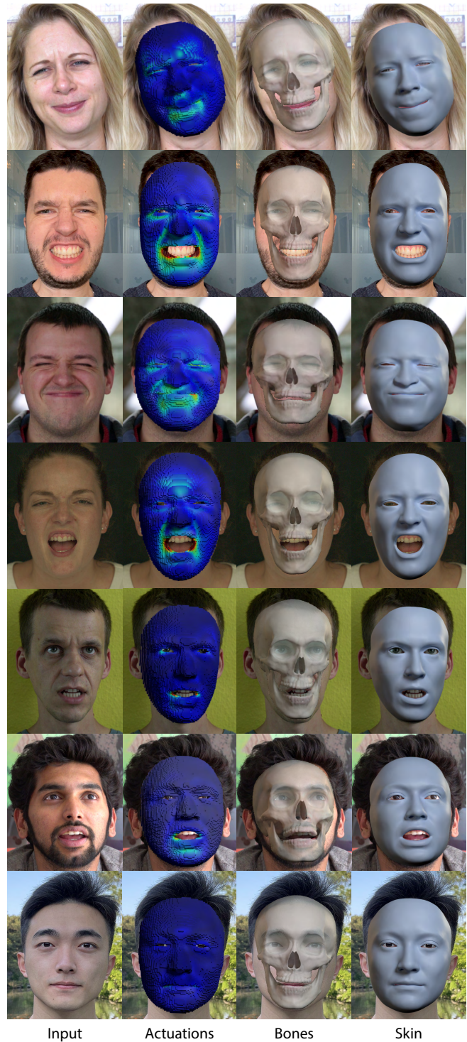
Fig. 5. Model fitting to a single face image. Seven different identities and expressions are shown. After fitting, the predicted actuations and bones allow to simulate the final facial skin mesh. The result is an animatable physical model from a very lightweight input.
