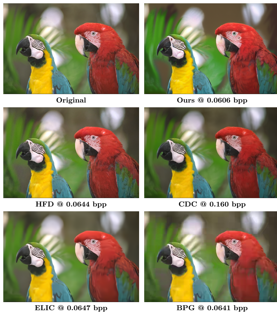
Fig. 22: Qualitative comparison of our method, HFD [25], CDC [46], ELIC [21], and BPG [1] on kodim23 . Best viewed digitally.
