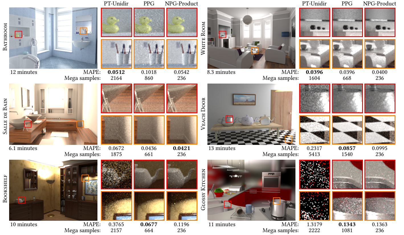
Fig. 15. Equal-time comparison of unidirectional path tracing (PT-Unidir), practical path guiding (PPG) [Müller et al. 2017], and our product-driven neural path guiding (NPG-Product). Despite the large computation cost of NPG, it performs competitively with PPG and outperforms unidirectional path tracing in scenes with difficult light transport (bottom two rows, sorted by difficulty in ascending order). The radiance-driven PPG algorithm tends to perform best because of its low computational cost, except when incident radiance is a poor approximation of the product (top row).
