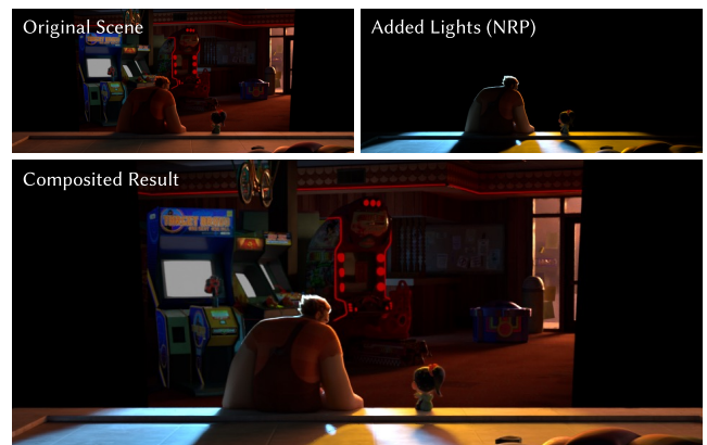
Figure 11: Compositing Application. Our NRP can be seamlessly combined with standard compositing workflows by training it for specific layers. In this Arcade example, an NRP is trained on the foreground layer only, allowing to relight it while leaving the background untouched. © Disney
