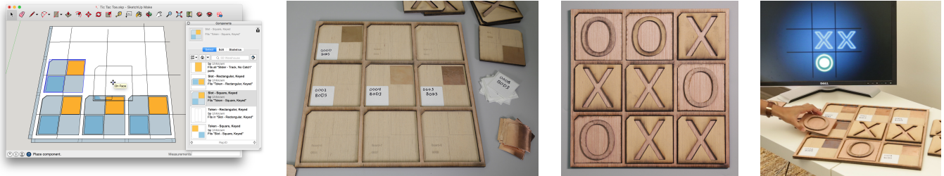
Figure 1. A wireless, batteryless game of Tic-tac-toe is designed using components in the RapID standard library, fabricated using laser cutting along with stick-on RFID tags and foil, and tracked with low latency using the RapID runtime library.
