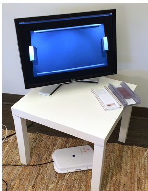
Figure 7. Our testing area consisted of an RFID antenna placed on the floor, a non-metallic table, and a monitor for visual feedback. The RFID reader and the computer running the application (both not shown) are placed to the side, and connected via ethernet.
