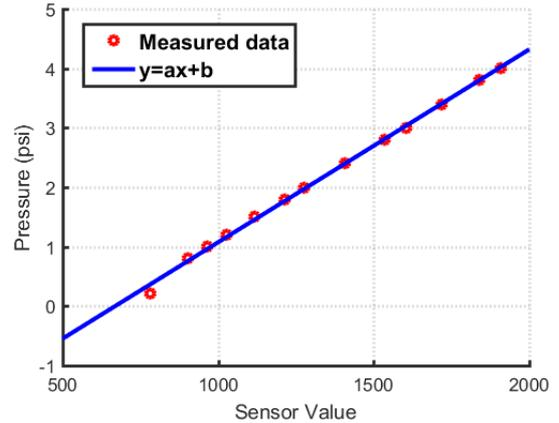
Fig. 5. Pressure sensor calibration plot. The relationship between the pressure sensor data and measured pressure is almost linear. We used the MATLAB polyfit function to get the coefficients:  $a = 0.0032$ ,  $b = -2.1704$ .
