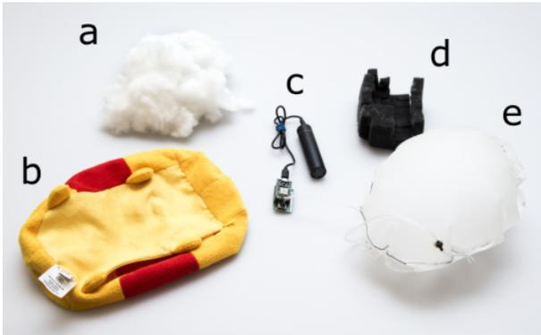
Fig. 4. Pressure data transmitting doll components including (a) stuffing, (b) fabric covering with zipper, (c) 3350 mAh battery, pressure sensor and Wi-Fi enabled microcontroller, (d) foam microcontroller housing and (e) heat-sealed polyurethane air bladder.
