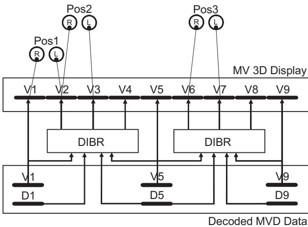
**Fig. 16.** Efficient support of auto-stereoscopic displays; Pos: viewpoint, R: right eye, L: left eye, V: view/image, D: depth.
