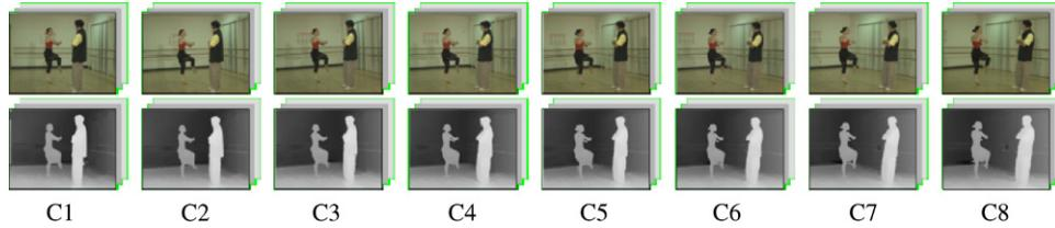
**Fig. 9.** Multi-view video plus depth. A scene is captured by 8 synchronized cameras (C1–C8) at the same time from different viewpoints. Depth is estimated for each of the camera views.
