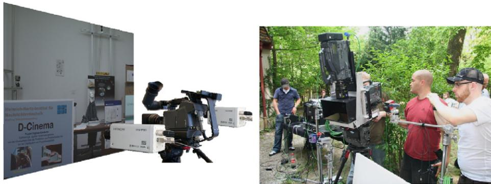
Fig. 5. Extended multi-view camera systems for 3DV and FVV acquisition.
