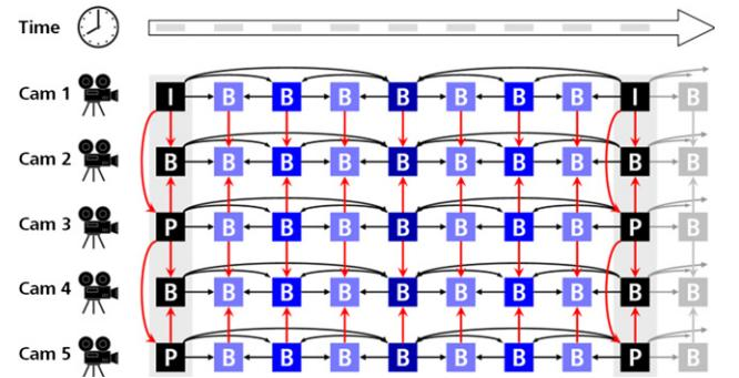
**Fig. 11.** Multi-view video coding (MVC).
