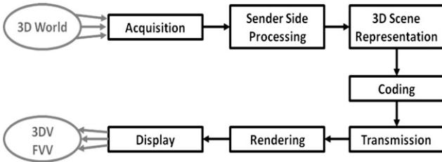
**Fig. 1.** 3DV and FVV processing chain from capture to display.
