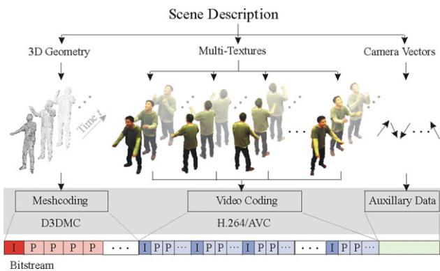
**Fig. 12.** Coding and multiplexing of dynamic 3D geometry, associated video textures and auxiliary data using MPEG-4 for model-based FVV.
