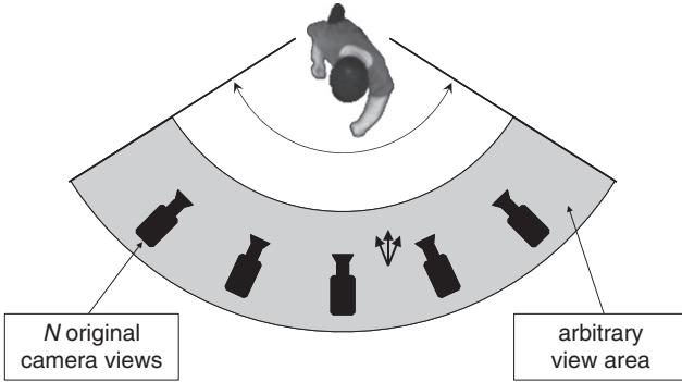
**Fig. 15.** Spatio-temporal video volume supported by MVD and LDV, given a certain camera setting.
