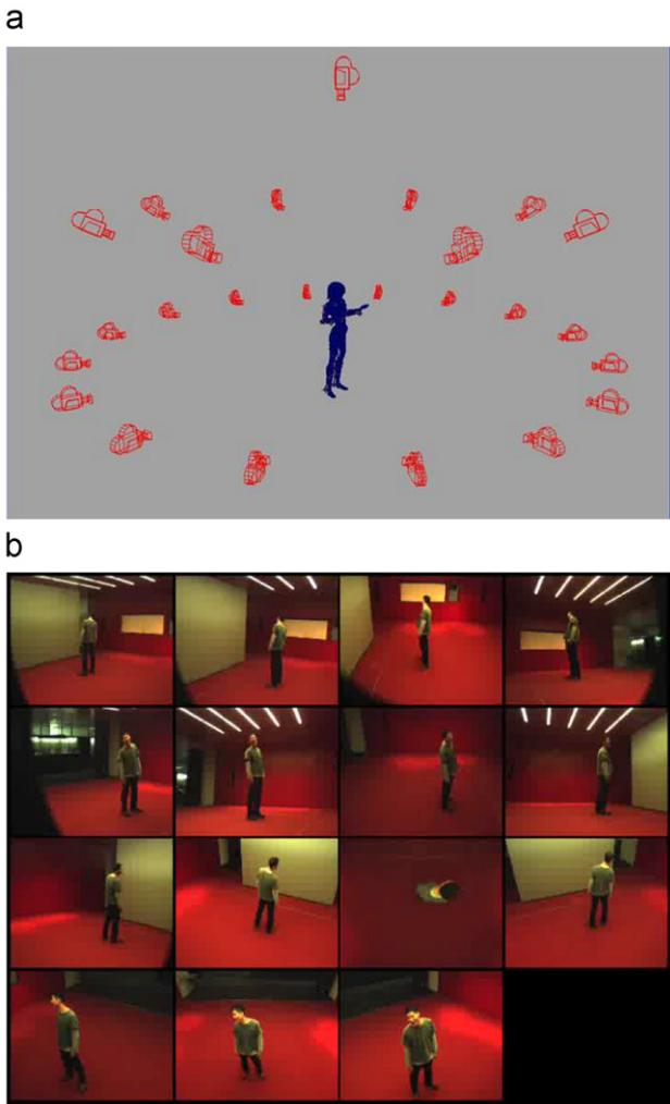
**Fig. 3.** Multi-camera setup for 3DVO acquisition and captured multi-view video.
