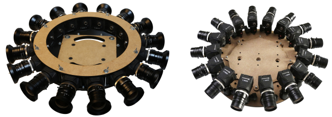
Fig. 9. Our two camera rig prototypes used for capturing panoramic content. The one on the left with a 3D printed camera mount has more accurate orientation and position of the cameras and lenses with a wider field of view compared to the hand-assembled rig on the right.
