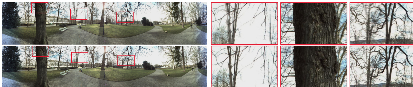
Fig. 14. The close-ups show that the panorama created with the depth based approach (top) contains considerably more ghosting artifacts than the panorama created with our flow-based approach (bottom).
