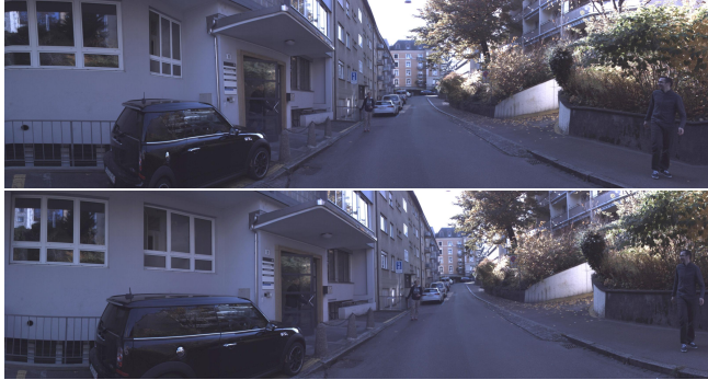
Fig. 11. Reconstructed panoramas without (top) and with (bottom) considering the extrinsic and intrinsic camera parameters. Note the significant, spatially varying distortion of the scene in the top image, such as the car and window. A consistent result as in the bottom is crucial, in particular for dynamic scenes and for plausible virtual head motion effects.
