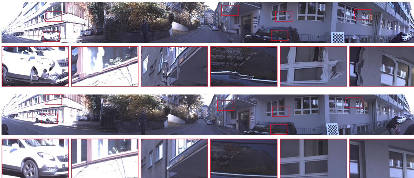
Fig. 16. The panorama created with Facebook’s Surround 360 algorithm (top) contains visible artifacts that are not present in our panorama (bottom). This is especially visible in the close-ups.
