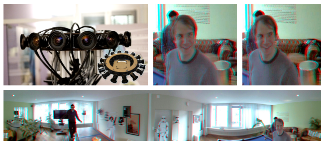
Fig. 1. Given videos acquired by a sparse camera rig (see our prototype with 16 cameras on the left), we describe a complete pipeline for the generation of high-quality stereoscopic omnidirectional videos of dynamic scenes (bottom), with support for smooth parallax interpolation between different viewpoints (two top right images), enabling real-time virtual head motion in Virtual Reality applications despite the sparse video input.
