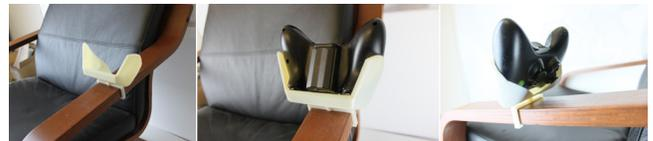
**Figure 16:** A connector that allows us to put a game controller to a chair arm.
