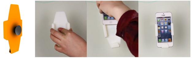
**Figure 13:** Mobile phone holder with a suction cup attaching to a glass plane. The top direction is specified as a free motion. Note that the whole thing including suction cup is printed.
