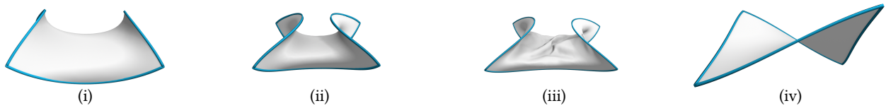
Fig. 2. The design space of KPS is highly nonlinear and the effects of parameter changes often difficult to predict. The images show a simple square frame ( 120 \times 120 mm) with different fabric pre-stretch factors s , normal rod width w_n (governing out-of-plane resistance), and binormal rod width w_b (governing in-plane resistance). From left to right: (i) ( s = 1.3 , w_n = 0.2 mm, w_b = 0.4 mm) base shape; (ii) ( s = 1.6 , w_n = 0.2 mm, w_b = 0.4 mm) higher stretch increases curvature; (iii) ( s = 1.3 , w_n = 0.2 mm, w_b = 0.2 mm) lower in-plane resistance leads to sagging and wrinkling; (iv) ( s = 1.3 , w_n = 0.4 mm, w_b = 0.4 mm) higher out-of-plane resistance leads to a completely different stable configuration.
