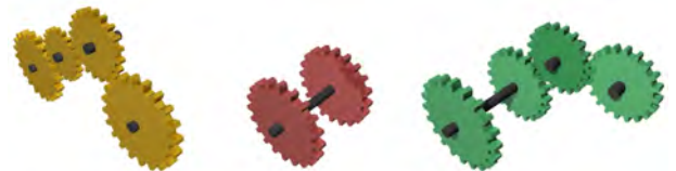
Figure 7: Types of connections generated during interactive gear layout: sequential (yellow), parallel (red), and combined (green).
