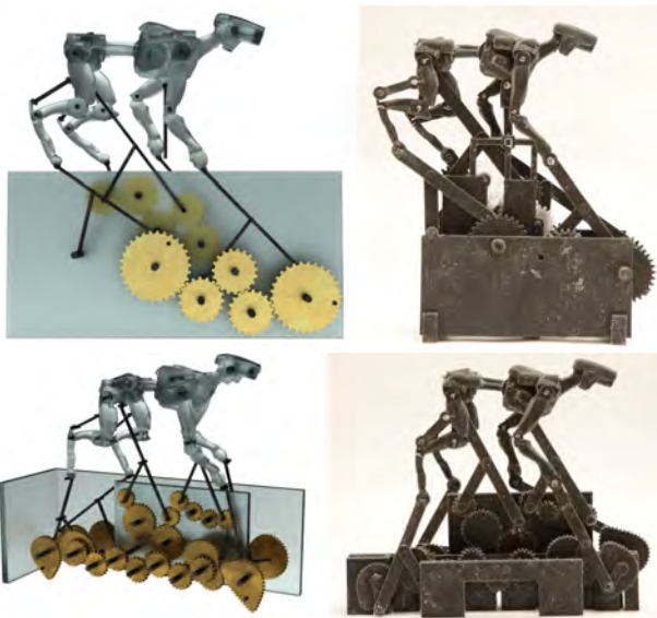
Figure 13: EMA Walk and EMA Gallop . For the galloping motion we use non-circular gears to control the timing of the foot-falls.
