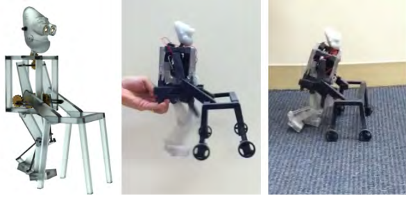
Figure 12: Bernie . A DC motor and a battery pack were added to the body to make the character walk on its own (with strings attached for support).
