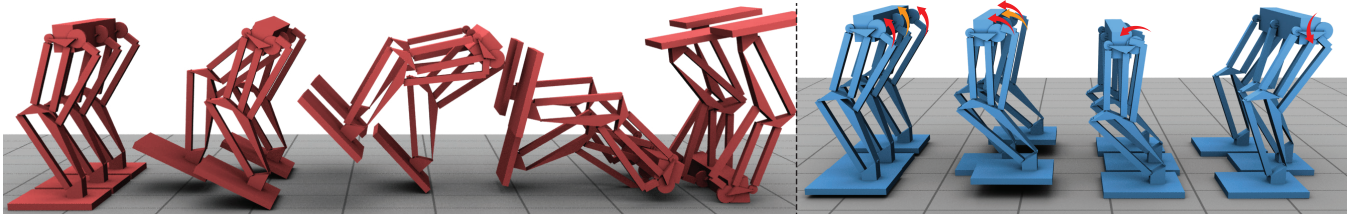
(b) Gorilla: A three-legged design with each leg alternating between support and swing-through phase.
