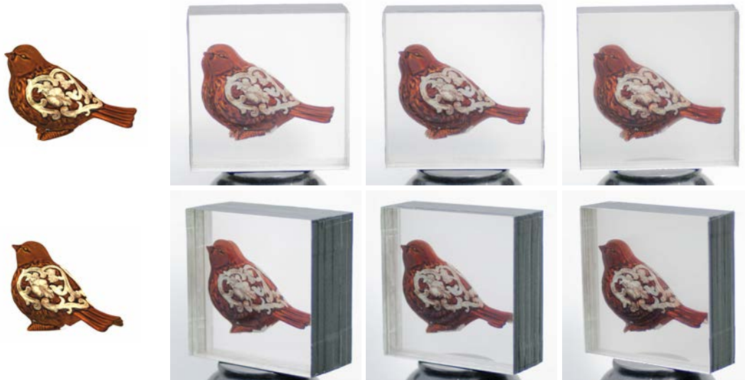
Figure 15: The input bird model (left) and the 5, 9, and 17 layer multilayer models (right) for two different views.
