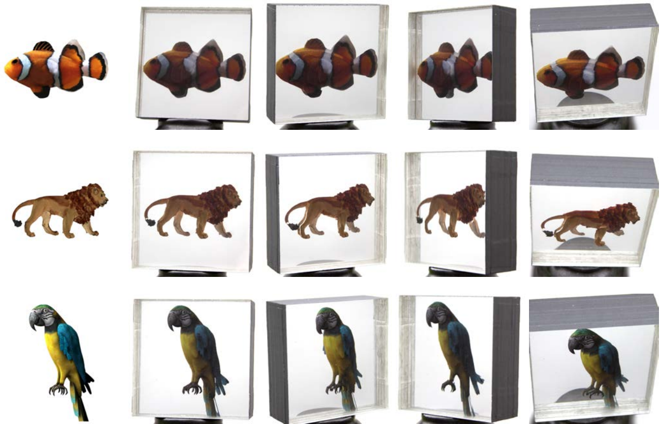
Figure 13: Left: Input model. Right: Four views of the corresponding 9-layer physical replicas constructed from lead-free glass.
