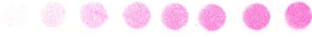
Fig. 5. Calibration samples of Prescale film, showing film color for contact pressures increasing linearly between 0.03 and 0.22 MPa.
