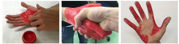
Fig. 2. Measuring contact area during a handshake. Paint is applied to the hand of one participant, a handshake is performed with a target participant, and the paint-transfer pattern on the target participant’s hand shows the contact area.
