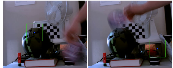
Figure 8: Motion blur is too severe in this scene for feature-based tracking to detect the object.
