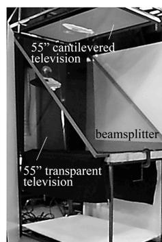
Figure 8. Setup for a 55" Pepper's Ghost with LCD mask.
