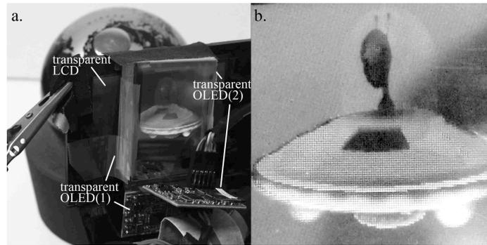
Figure 13a,b. Images of dual-layer transparent OLED with LCD mask.
