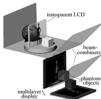
Figure 4. Setup of beam-combiner with multilayer display and LCD masks.
