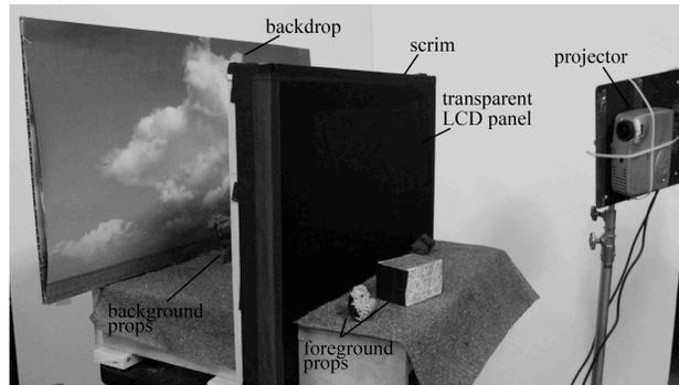
Figure 6. Setup of scrim projection with LCD mask.
