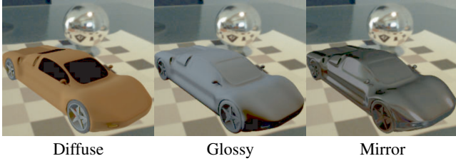
Figure 4: Shading, including soft shadows, from global/ambient light (directional light omitted) due to each BRDF component (> 70 FPS).
