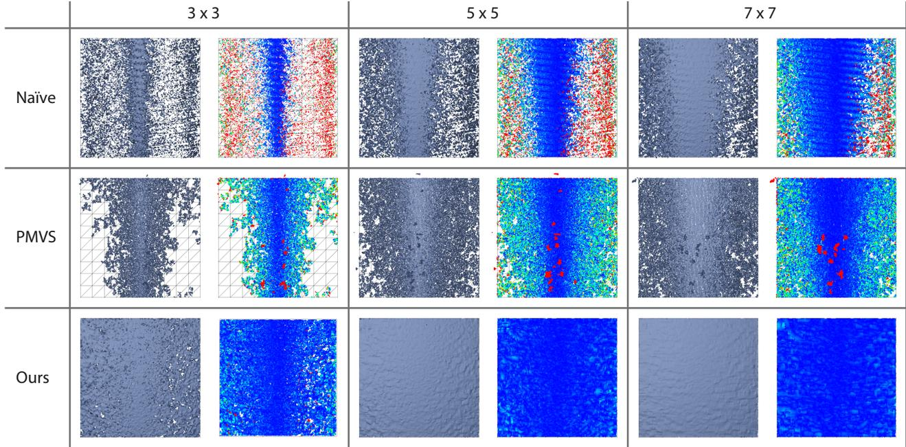
Figure 7. **Qualitative Evaluation** - Rendered point cloud results and error maps for the evaluated algorithms at three different window sizes. The error maps encode Euclidean distance to the plane in a rainbow scale, running from blue (low error) to red (high error).
