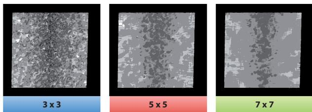
Figure 8. **Match Levels** - Visualizing the matching level for each pixel at three different window sizes. Darker areas correspond to matching at lower levels. For smaller window sizes the frequency content varies more between patches, leading to a wider spread in matching levels.
