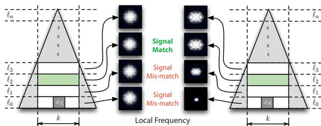
Figure 5. **Equalization Algorithm** - We continually traverse up the scale-space of two images centered on  $x_L$  and  $x_R$ , respectively, until the local frequency signals are equalized and optimal for correspondence matching.
