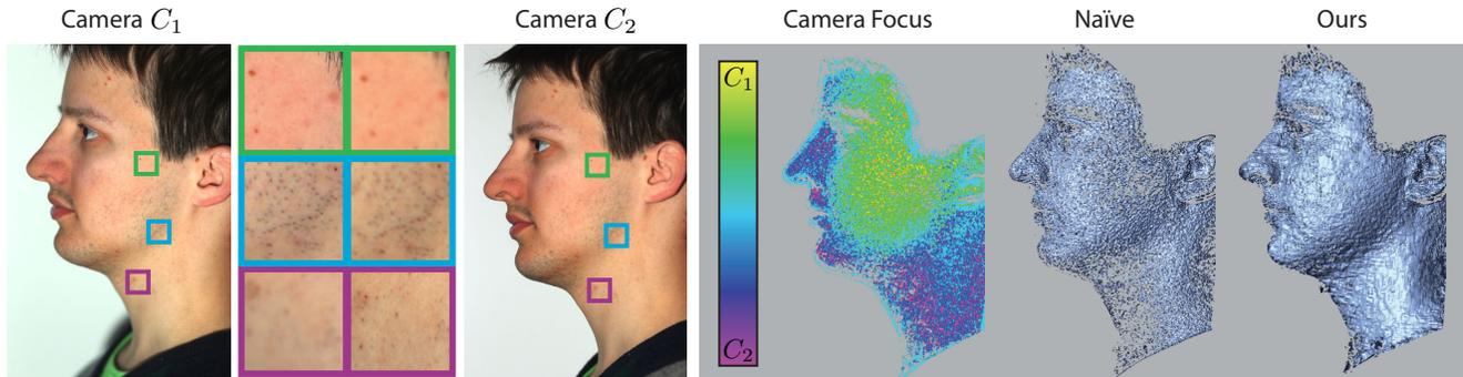
Figure 9. **Real-world Face Example** - *Left*: The images from cameras  $C_1$  and  $C_2$  have different focal planes with limited depth of field. *Center*: Color-coded difference of local frequencies. *Right*: 3D point cloud results. The naive algorithm successfully reconstructs areas where the signals are similar but quickly degrades with increasing signal mismatch. Signal equalization greatly improves accuracy and robustness in areas of signal mismatch.
