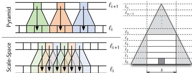
Figure 4. **Scale-Space** - *Left*: Image pyramids have an ambiguity in the parent-child relationship which is resolved by a complete scale-space. *Right*: For efficiency, we store only slices of the scale-space which are computed on-demand.
