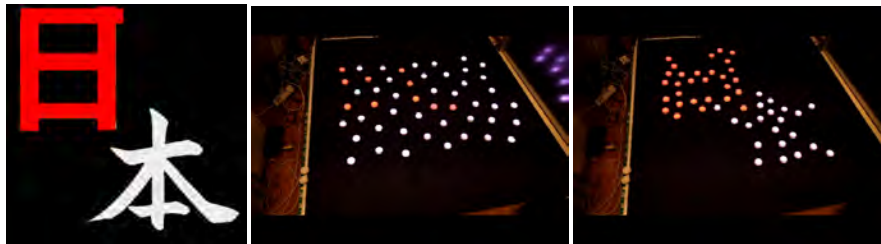
Fig. 9 Illustration of the bottleneck problem. At left , the user drawing. At center , robot start position. At right , the shape is convoluted, and diffusion of robots to achieve the shape is slow.
