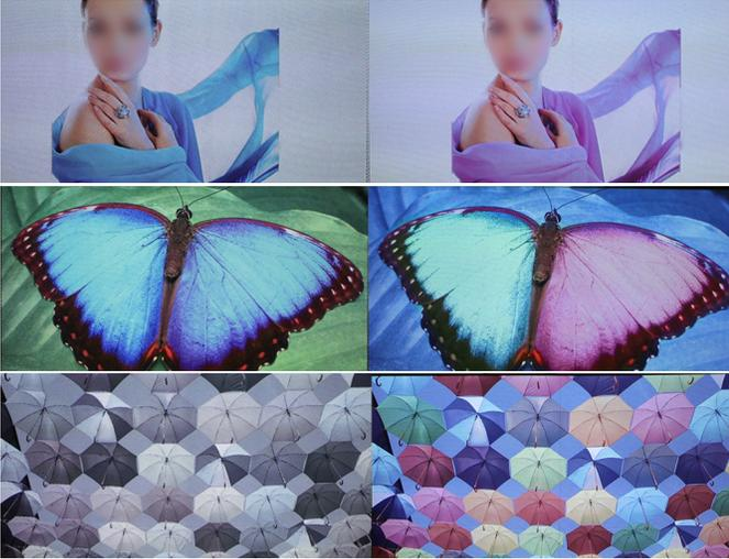
Fig. 6: Photographs of hue and chroma alterations. Left: Projection onto *pattern surface*. Right: The same projection onto the *white surface*. The upper row shows a slight hue shift of  $45^\circ$ . The center row more drastic hue shifts and in the bottom row a chroma change example is shown. (All images are taken with automatic aperture and white balance.)
