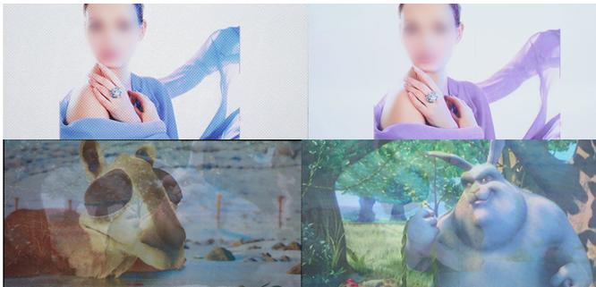
Fig. 15: Photographs of Image-based approach: the left side shows projection onto the *b/w pattern surface*. On the right, the same projection is shown on a *white surface*. (All images are taken with automatic aperture and white balance.)
