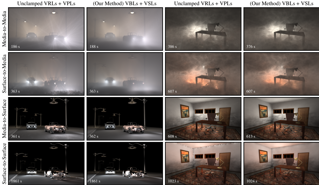
Figure 9: We isolate and visualize the four different transport paths in the CARS (left half) and SMOKYROOM (right half) scenes. We compare our VBL+VSL method (second column in each set) to unclamped VRLs+VPLs [NNDJ12] at equal-time.
