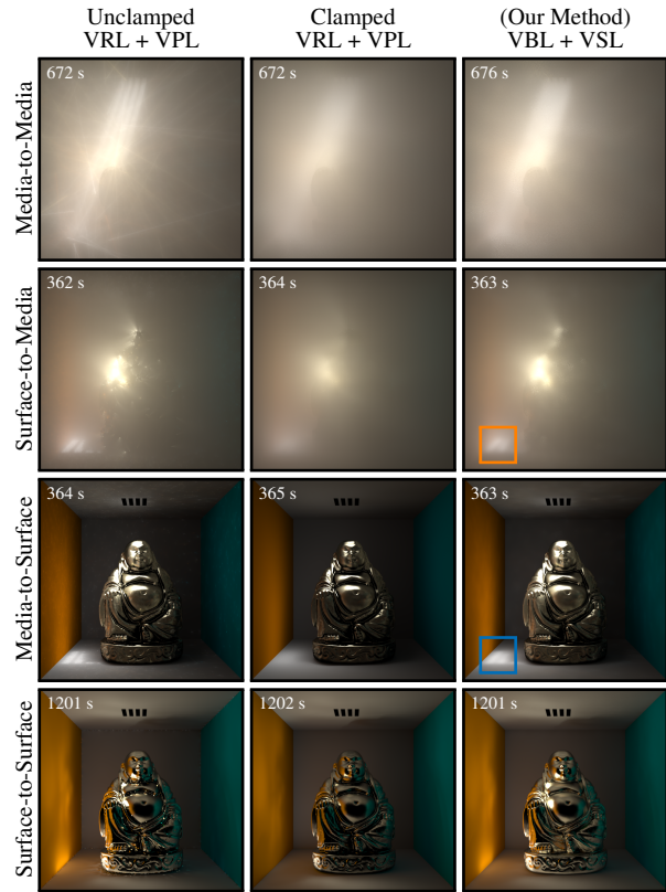
Figure 7: An equal-time (unconverged) comparison in the BUDDHA scene between unclamped/unbiased VRLs+VSLs (left), clamped VRLs+VSLs (center), and our method (right).
