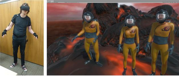
Figure 15: Avatars in an video game engine VR environment with live body motion capture using a Perception Neuron IMU based motion capture system.
