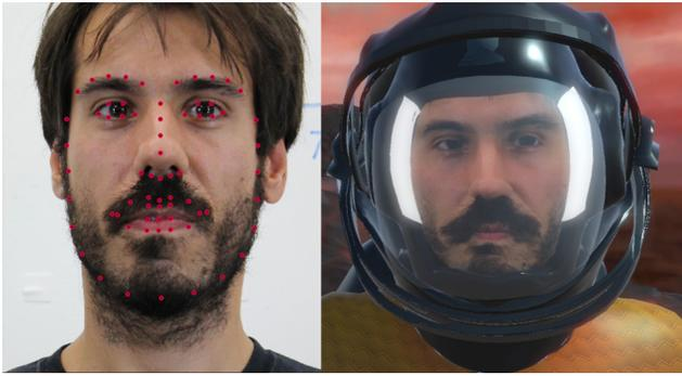
Figure 14: Face fitting failure case - poorly detected mouth landmarks causing the mouth to be misaligned avatar.
