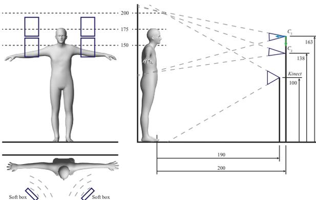
Figure 3: Avatar capture hardware configuration. The rectangles depict illumination soft boxes,  $C_1$ ,  $C_2$  and *Kinect* are capture devices.
