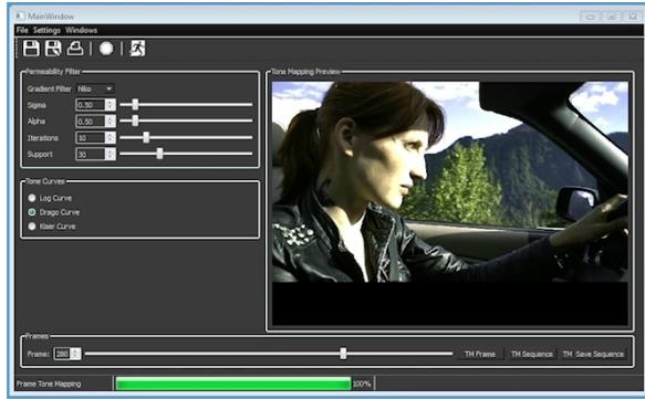
**Fig. 4.** The graphical user interface of our prototype implementation. Users can change parameters of the permeability guided filtering as well as the tone curve. Parameters can be set on a desired number of key frames, which our system then applies to the entire video sequence by interpolation. All changes are reflected at interactive rates through a rendering of the currently selected frame that is tone mapped using the desired parameters.
