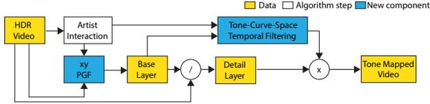
**Fig. 2.** Real-time HDR video tone mapping workflow with the proposed modifications to the previous state-of-the-art. See text for details.
