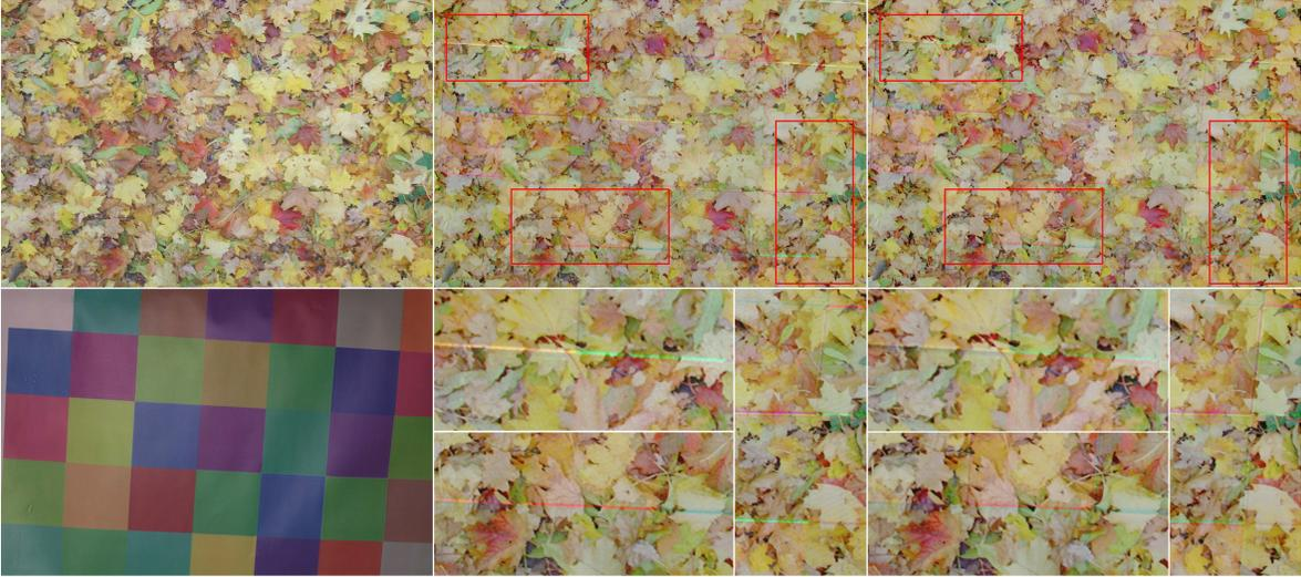
Fig. 4: Comparison of a drift optimized compensation (right) with a conventionally compensated projection (center) in a misaligned projection setup. The input image is shown in the upper left, the lower left shows the projection surface containing hard edges. The other images in the lower row show close ups of the regions highlighted in red. Note that the hard color seams are visually reduced with our approach.
