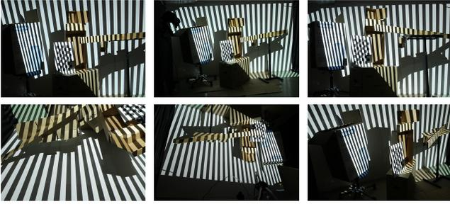
Figure 6: The six camera views for dataset #11. Even though the structure of the scene is rather complex including several reflections, our self-calibration procedure manages to successfully calibrate all devices within less than 4 minutes.
