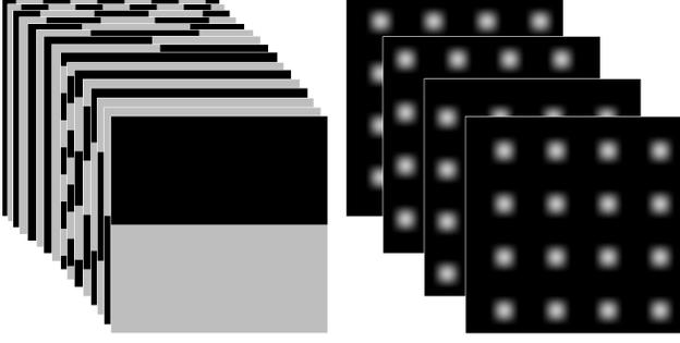
Figure 1: A simplified structured light pattern sequence to generate sub-pixel accurate correspondences between the devices. Complementary Gray codes are used to reliably generate coarse references. The additionally projected blob patterns are then used to refine them down to sub-pixel accuracy. Depending on the application requirements, all, or only a subset of all projector pixels, are used for correspondence generation.
