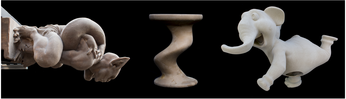
Fig. 1. We optimize the strength-to-weight ratio and mass distribution of binder-jetted, large-scale structures under worst-case loads, in order to make them durable (left, middle, right) and stand (right). Given a combination of live, wind, dead, and thermal loads common in structural engineering, our optimization identifies worst-case wind directions and contact regions, minimizing resulting peak stresses.
