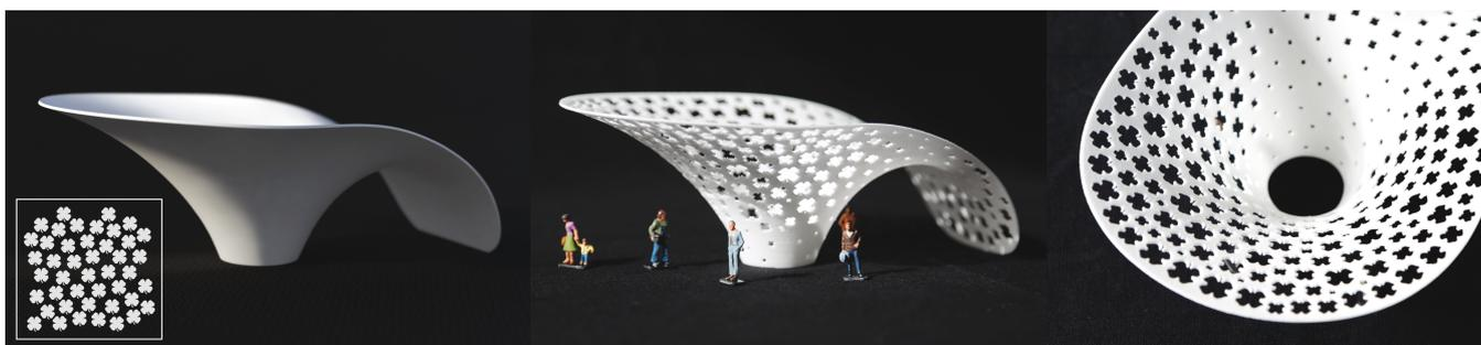
**Figure 1:** Our design tool allows users to create physical surfaces structured with decorative patterns. Given a base shape and pattern exemplar (left), our method creates a distribution of stencils that are used to remove material from an otherwise solid surface. The result (center, right) is a physical surface that combines user-controlled aesthetics and structural integrity.
