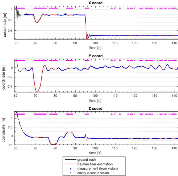
Fig. 9: Comparison of the estimated cavity position, the measured cavity position from the vision-based detection and the ground truth in frame  $\mathcal{V}$  during the simulation experiment.
