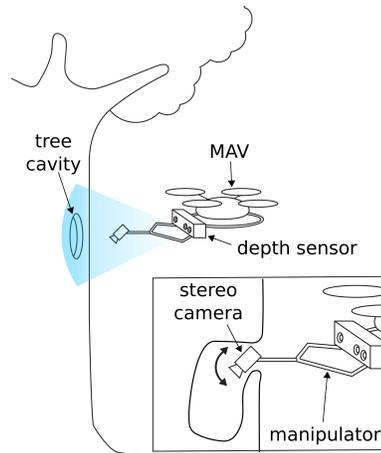
Fig. 1: A MAV equipped with a dexterous manipulator performing a tree cavity inspection using a depth sensor to detect the cavity and a close-up view of the end-effector of the manipulator fitted with a stereo camera being inserted into a cross section of the cavity.
