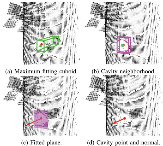
Fig. 5: Point cloud from a simulated detection sensor, showing a tree cavity and the different processing steps performed to refine the detection of the 3D position of the cavity and compute its normal.
