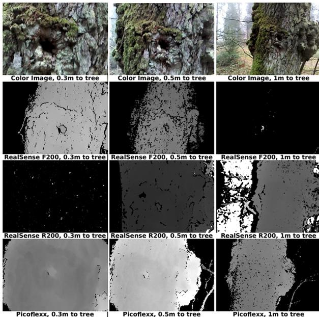
Fig. 7: Comparison of depth images acquired by the Intel RealSense Camera F200 (2nd row), Intel RealSense Camera R200 (3rd row) and pmdtechnologies CamBoard pico flexx (4th row) of the same tree cavity at approximately 0.3m (1st column), 0.50m (2nd column) and 1m (3rd column) while mounted on a telescopic pole on a field trip in the forest . The first row shows a color image of the cavity taken at the corresponding distance from the tree.
