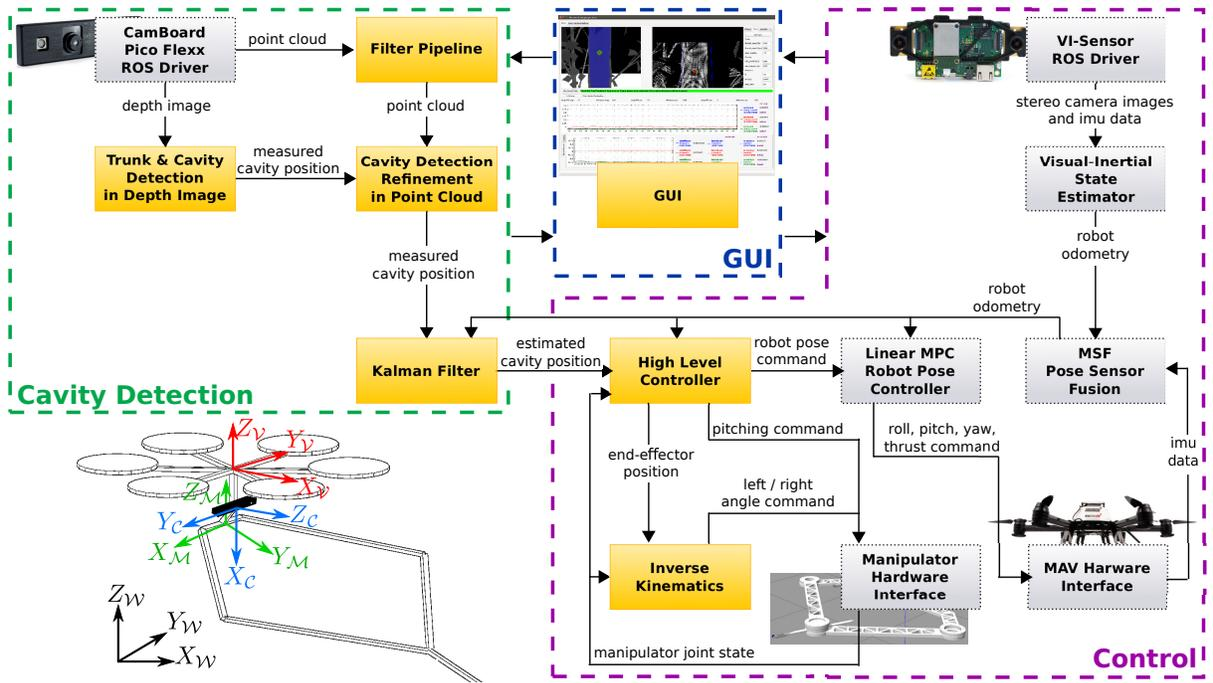
Fig. 3: The software architecture and the defined coordinate frames for the system.
