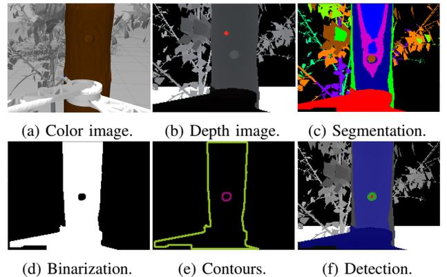
Fig. 4: Simulated color image and depth image from a simulated detection sensor, showing a tree cavity and the different image processing steps performed to detect the 3D position of the cavity.
