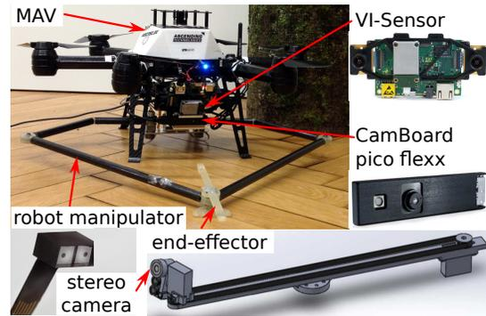
Fig. 2: The hardware comprised of an AscTec Neo hexacopter MAV, a VI-Sensor, a CamBoard pico flexx time-of-flight 3D camera, a parallel robot manipulator and an end-effector fitted with a NanEye stereo camera, an LED light, a laser and servo motors.
