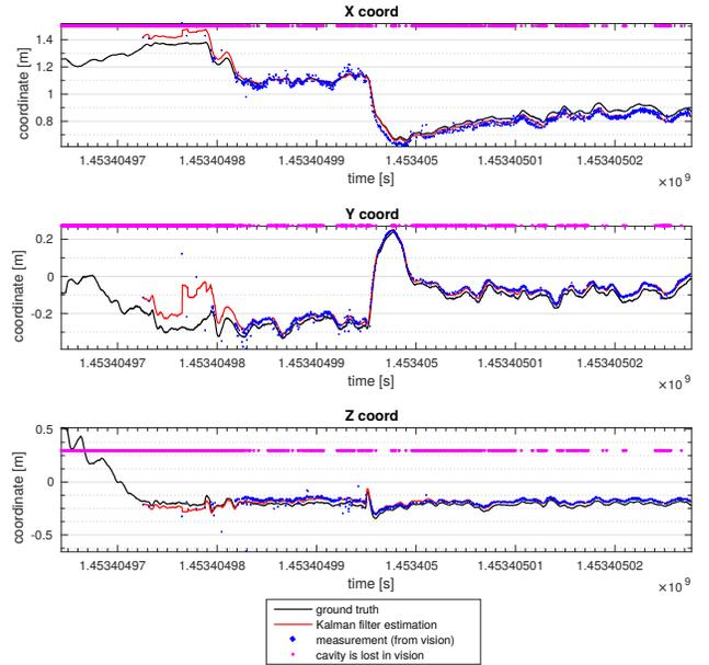
Fig. 11: Comparison of the estimated cavity position, the measured cavity position from the vision-based detection and the ground truth in frame  $\mathcal{V}$  during the real-world experiment.
