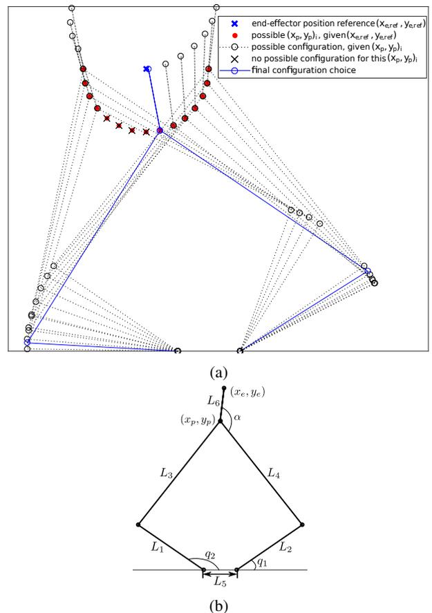
Fig. 6: The manipulator configuration and a visualization of the inverse kinematics process for a planar delta manipulator with an end-effector.
