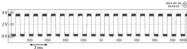
Figure 9: Oscilloscope snapshot of light intensity output of a modified light bulb in idle mode, the light is duty-cycled at 50 %.
