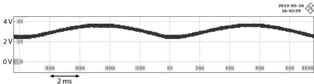
Figure 8: Oscilloscope snapshot of the light intensity output of an unmodified light bulb. The figure shows the typical pattern of an AC/DC power supply.
