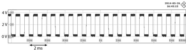
Figure 9: Oscilloscope snapshot of light intensity output of a modified light bulb in idle mode, the light is duty-cycled at 50 %.
