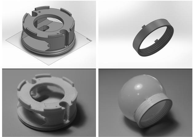
Figure 6: 3D-model and 3D-printed additional light bulb parts. Left: mounting to create additional room for the microcontroller, right: ring with internal thread attached to the plastic cap to securely close the light bulb again.
