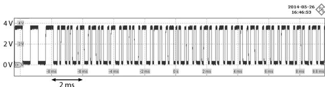
Figure 10: Oscilloscope snapshot of light intensity output of a modified light bulb while transmitting data.
