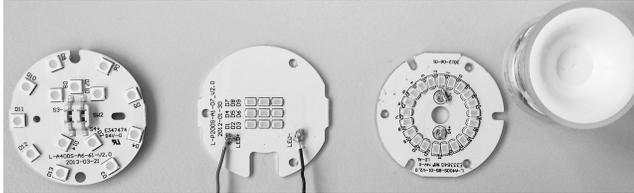
Figure 3: LED boards of the three consumer LED light bulbs, no. 1 to 3 from left to right.
