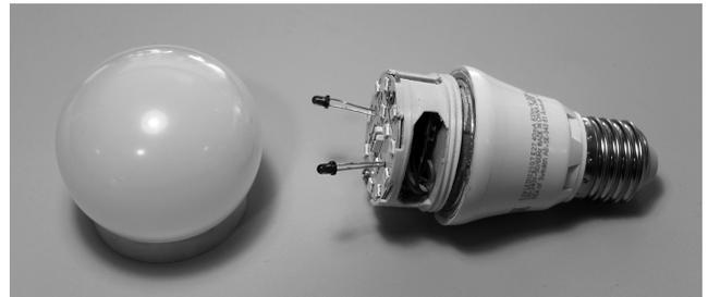
Figure 7: Assembled smart LED light bulb with unscrewed cap and connected phototransistors.
