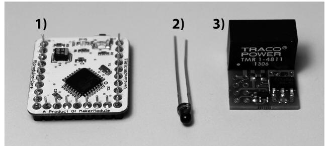
Figure 5: Additional electronics added to the consumer LED light bulb. 1) microcontroller board, 2) phototransistor, 3) custom designed power conversion PCB.
