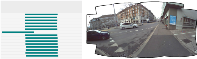
Figure 11: By finding relative temporal offsets of clips from a 15 camera array (left), it becomes possible to construct a video panorama without ghosting on moving objects (right).
