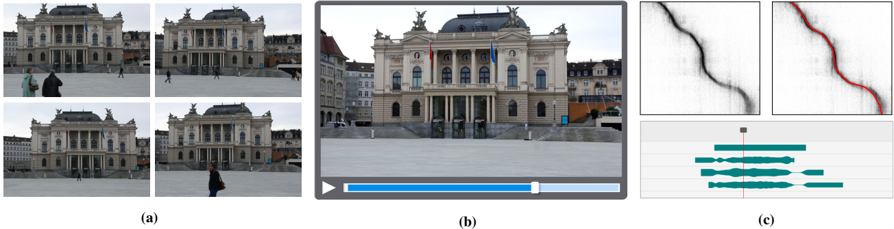
Figure 1: Four videos are taken of the same scene at different times from roughly similar camera trajectories (a). Spatiotemporal alignment greatly simplifies complex video editing tasks. Here, we removed the people from all video clips with a simple median filter (b). Our method efficiently finds a nonlinear temporal warping, synchronizing multiple videos by computing paths in a cost matrix (c) above. This is visualized by the squeezing of clips in the timeline (c) below, resulting in an intuitive, interactive video alignment tool.
