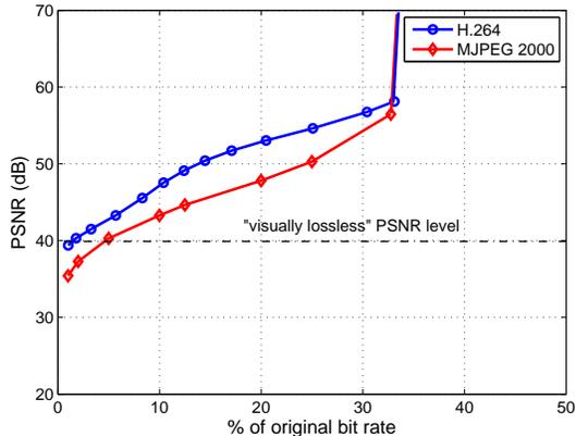
Figure 4. The impact of compression on video quality. H.264 and MJPEG 2000 are able to compress the test sequence to, respectively, 1% and 5% of its original bit-rate while keeping the PSNR at the visually lossless level.
