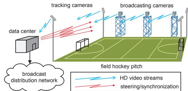
Figure 1. The microcasting system relies on tracking cameras to transmit information about the action to the central data processing center. This information is used by computer vision algorithms for automated decision making in the data center, which transmits the resulting control information to steer the broadcasting cameras. Video streams from the broadcasting cameras are sent to the data center where the final broadcast content is produced and forwarded to the content distribution network.
