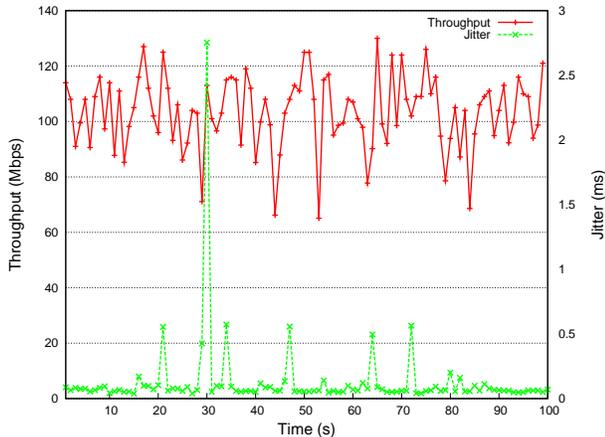
Figure 5. Throughput and delay jitter over a link with two nodes in proximity. For the test we use 802.11n WLM200NX Atheros chipsets with open-source Ath9k driver and place the node in proximity. Results show that throughputs of around 100 Mb/s are possible using commodity hardware with high flexibility for research scopes. The plot also shows that the delay jitter is mostly below 0.1 ms.
