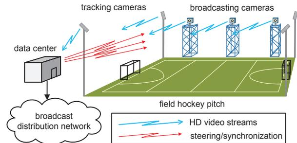
Figure 1. The microcasting system relies on tracking cameras to transmit information about the action to the central data processing center. This information is used by computer vision algorithms for automated decision making in the data center, which transmits the resulting control information to steer the broadcasting cameras. Video streams from the broadcasting cameras are sent to the data center where the final broadcast content is produced and forwarded to the content distribution network.
