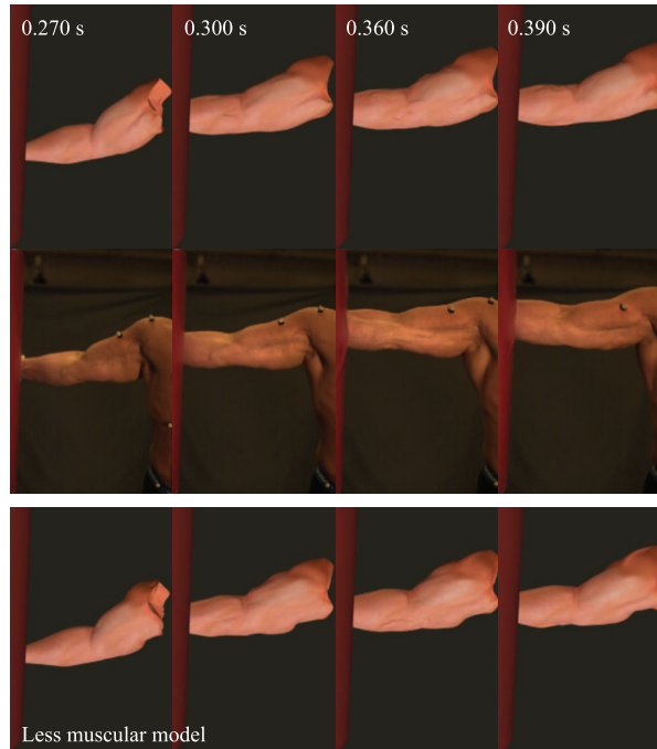
Fig. 8 Skin deformation simulation of an arm with an external impact. The bottom row shows a simulation result with a less muscular model.
