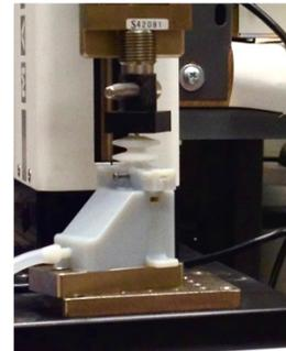
Figure 7 - The experimental setup used for performing force-displacement tests. Bellows are mounted onto a removable test jig and measured for spring deformation.
