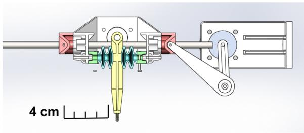
Figure 5 – A cross sectional view of the VSA. The PDMS bellows (blue) may be inflated to exert force onto the output link (yellow). A DC gear motor creates reciprocating linear motion of the carriage.
