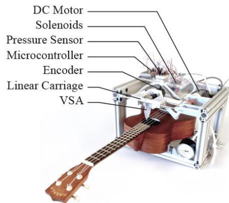
Figure 4 – An annotated image of a softly strummed ukulele using a VSA.
