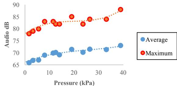
Figure 11 - Measured audio decibel intensity with respect to changes of the VSA's spring stiffness.
