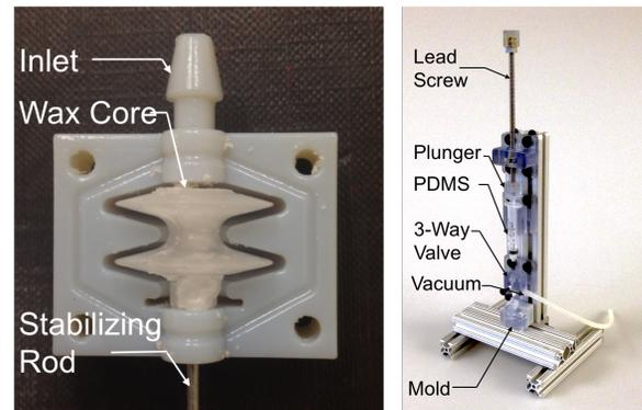
Figure 3 - (left) A wax core centered within the PDMS cast, ready for injection molding. (right) A leadscrew-driven injection molder having a 3D-printed three-way valve for degassing molds prior to injecting PDMS.
