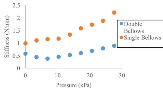
Figure 8 – A double and single bellows' spring constant from a linear fit of force-displacement data.
