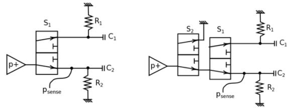
Figure 6 - (left) The pneumatic circuit configuration for position control. (right) A pneumatic circuit for stiffness control, with  $S_1$  held at 50% PWM duty cycle.
