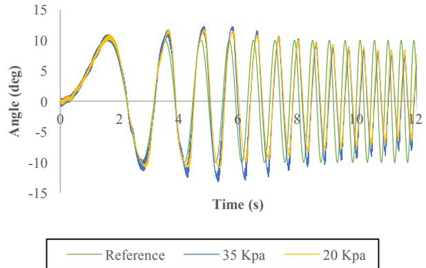
Figure 10 - Positional accuracy as a function of input pressures 35 kPa and 20 kPa. At higher frequencies, positional error is exaggerated with lower operating pressures.
