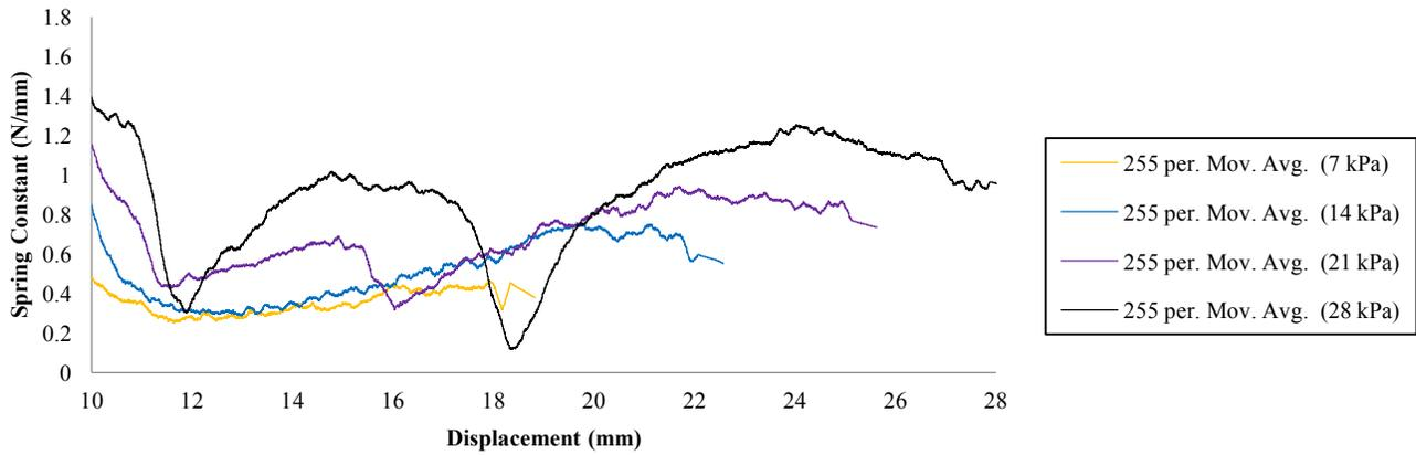
Figure 9 - Calculated spring constants when performing a force-displacement test on a double bellows. At higher pressures, the double bellows buckled under load, as reflected in the graph's deviations.
