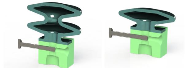
Figure 2 – (left) An illustration of a double stage bellows assembled into a pneumatic low-pass filter base. (right) A single bellows configured into the same base.
