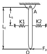
Figure 1 - A free body diagram of a revolute VSA having two antagonistic linear springs to provide stiffness at the output of link A.
