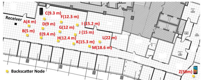
Fig. 9. In our experiments, the UBR was placed in a fixed location denoted by the black square; the backscatter node was moved to 14 different locations denoted by the yellow markers. A mobile phone was placed at locations C and Z to measure the contribution of cellular uplink channels.
