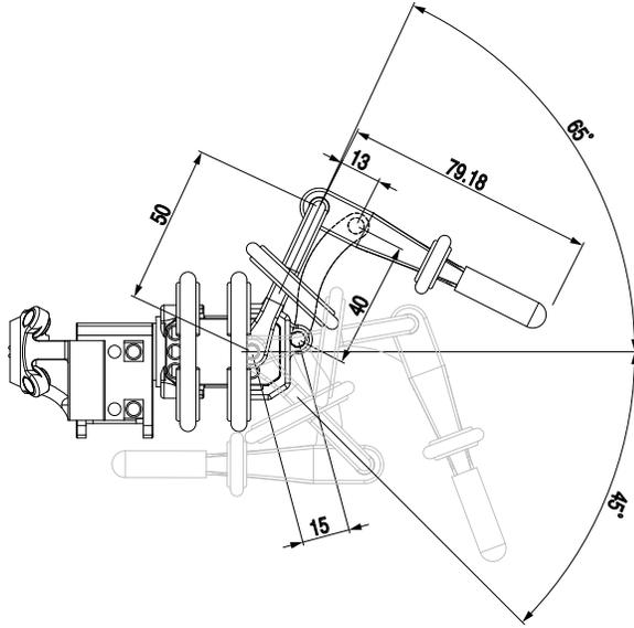
Fig. 5. Roll-Pitch Leg. Each leg has two to three position-controlled servos (roll, yaw, pitch) which are linked via snap-together 3D printed frame components. The four-bar linkage driven by the pitch servo creates a step-like foot trajectory. All units in (mm).
