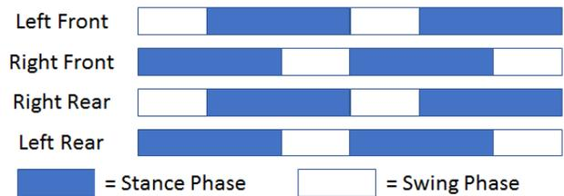
Fig. 9. Ground contact visualization of two walking cycles in trot gait
