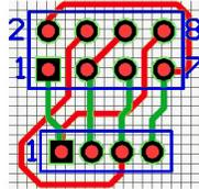
Fig. 4. The small PCB connects the coupling’s electrical connector to the 4-pin connectors enabling power and data to transmit in two 180° offset configurations.
