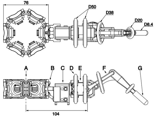
(b) Drawings of Body and a Roll-Pitch Leg
