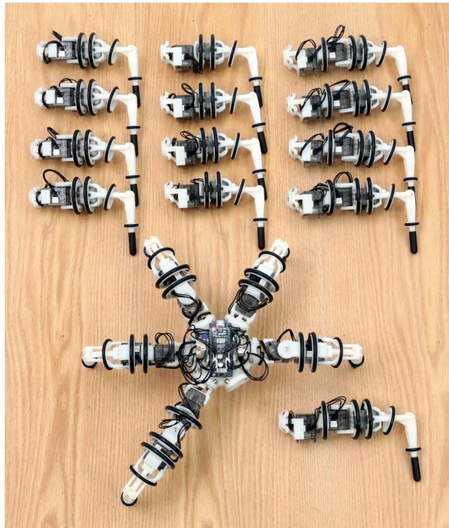
Fig. 1. Snapbot can have up to six legs at a time. There are three types of magnetically coupled removable legs; six each. A locomotion algorithm determines the robot’s configuration in real-time and chooses a combination of motions to propel the robot on a forward path.
