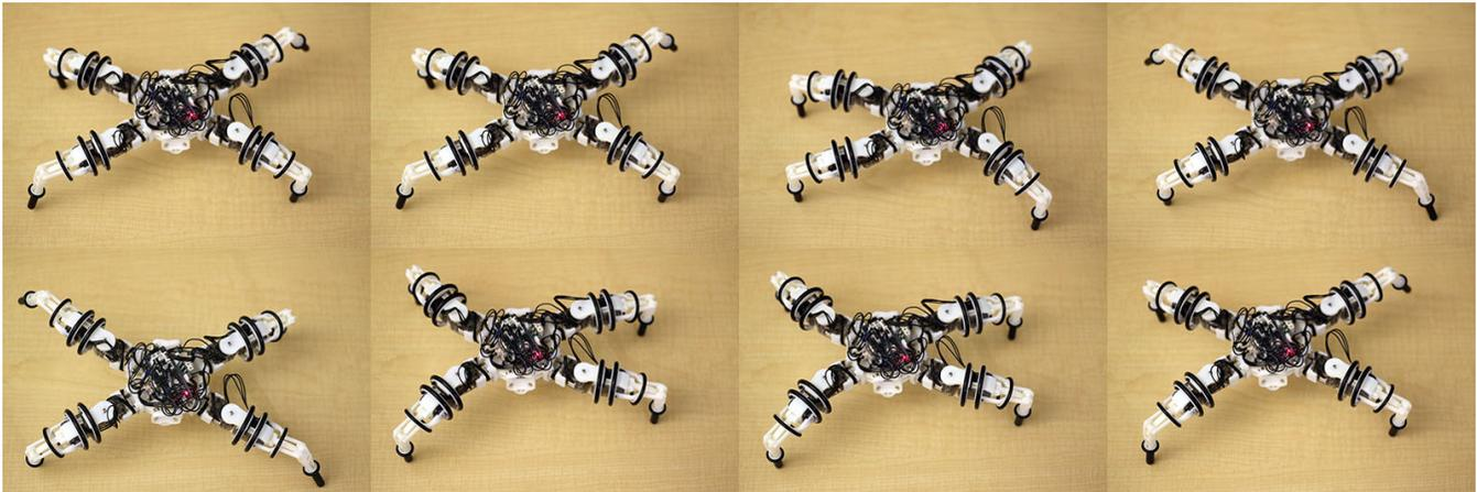
Fig. 10. Series of pictures of four legged walking. Snapbot is moving towards the top of the page (upward) using a trot gait. All attached legs are yaw-pitch legs. Pictures were taken every 0.1 sec and the order is from left to right, top to bottom.
