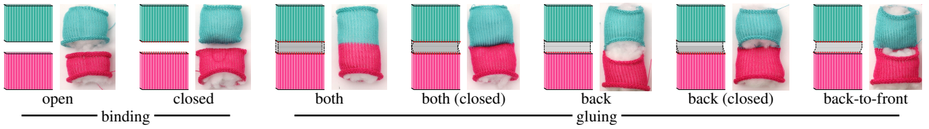
Figure 6: In our compiler’s input, each primitive has a start and end boundary definition that indicates how to stabilize loops. These can result in primitives that are open, closed, or attached together in various ways. Not shown are front, front (closed), and front-to-back gluing, which are defined analogously to their back variants.
