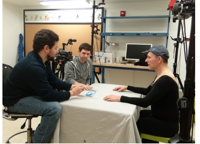
Fig. 2. The setup used for the synchronized Kinect and OptiTrack based head motion capture. The actor interacted with two subjects while performing the tasks to ensure that his gestures are natural.
